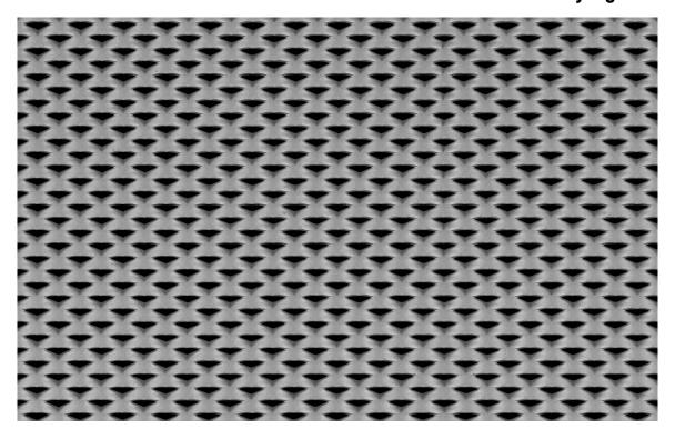
LW Pitch:10.00mmStrand Width:2.45mmSW Pitch:6.09mmThickness:1.50mmWeight:9.47 kg / m2Open Area:19%
